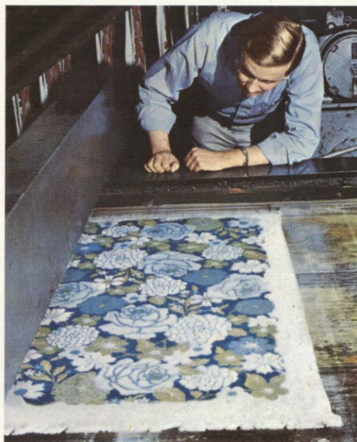
Grants' toweling quality-checked on the loom
